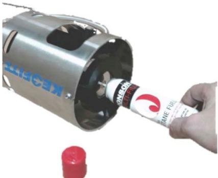
A hand is shown connecting a white gas cylinder to the burner of a silver sterilizer. A red cap is shown separately below. |
